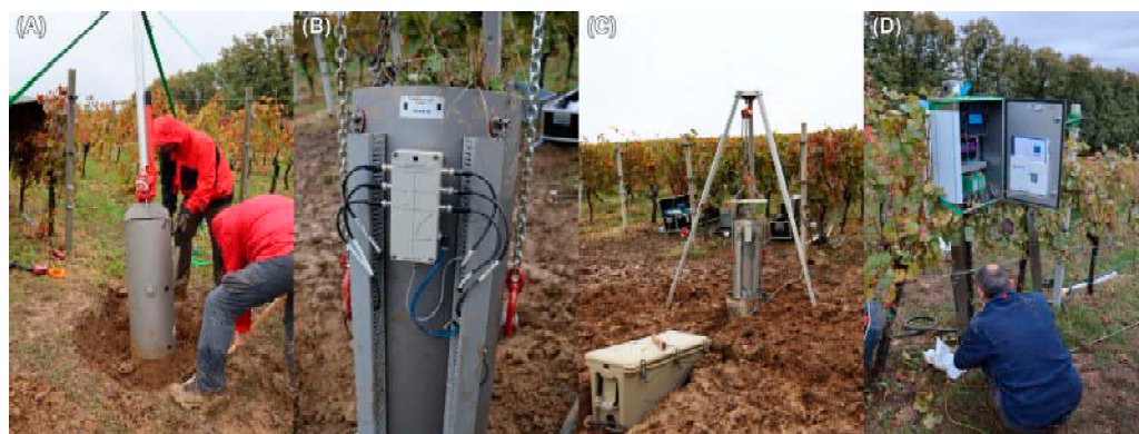
Figure 3. Installation procedure of the high-precision weighing lysimeter system at the SUPREHILL CZO: (A) vertical downpress of the cylinder during excavation; (B) connection of the sensors and system parts; (C) lowering of the cylinders below ground level and placement of the drainage tank (field box); (D) installation of the central control unit.
